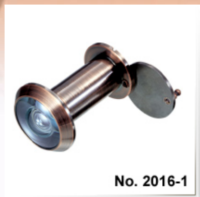
2016-1 DOOR VIEWER Synthetic Lens With Incorporated Cover Angle: 200 Degree Tube Dia.: 16mm & Outside Dia.: 30mm Fit Door Thickness: 35mm-55mm
